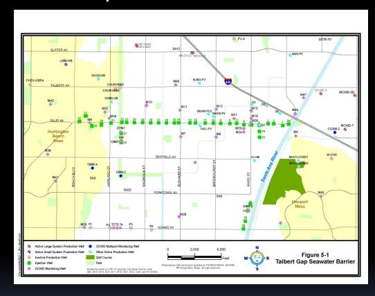
The Talbert Barrier consists of 36 injection well sites that recharge multiple aquifer zones to prevent seawater intrusion as well as to replenish the groundwater basin. Active since 1970's. Operates now at 20 to 36 MGD (75K – 136K m³/day).
