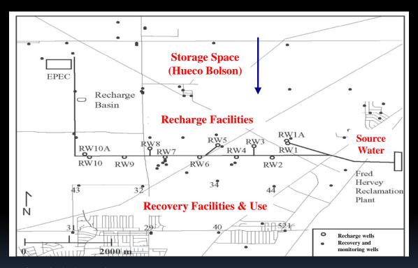
MAR facilities includes 10 recharge wells constructed in 1984 and one recharge basin built in 2001. Flow rate up to 10 MGD (38,000 m<sup>3</sup>/day)
