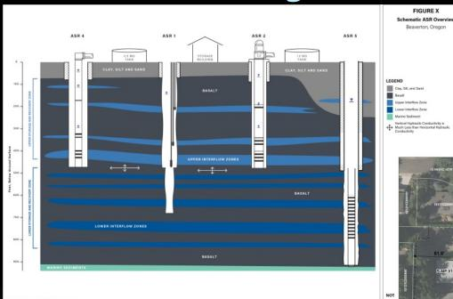
Recharge and recovery from interflow zones in continental basalt flows; Completed in 2001 and 2005; Peak flow = 5 MGD
