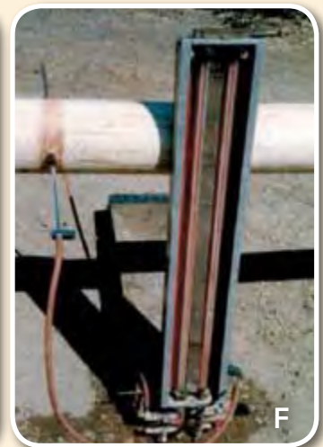
Figure 1: Various discharge measuring devices: (A) 5-gallon bucket and stop watch – Mulegé, Baja California Sur, Mexico; (B) Pipe and circular orifice – Sumner, WA; (C) in-line flow meter – Petaluma, CA; (D) in-line flow meter – Livermore, CA; (E) variable area flow meter – Minden, NV; and (F) differential pressure flow (velocity probe 9 ) meter using Pitot tubes and manometer – Healdsburg, CA.
