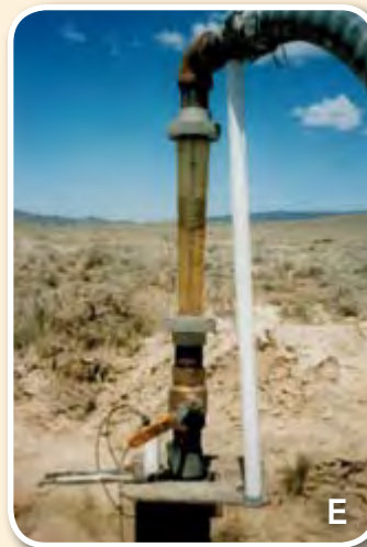
Figure 1: Various discharge measuring devices: (A) 5-gallon bucket and stop watch – Mulegé, Baja California Sur, Mexico; (B) Pipe and circular orifice – Sumner, WA; (C) in-line flow meter – Petaluma, CA; (D) in-line flow meter – Livermore, CA; (E) variable area flow meter – Minden, NV; and (F) differential pressure flow (velocity probe 9 ) meter using Pitot tubes and manometer – Healdsburg, CA.
