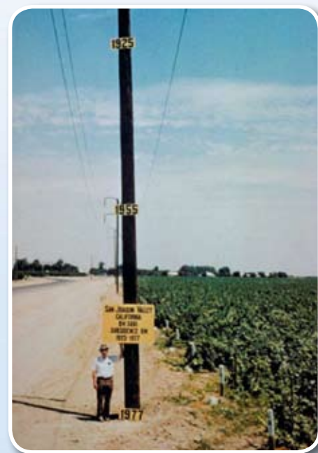
Figure 1. Approximate location of the maximum measured subsidence in the San Joaquin Valley, near Mendota, California. Land surface subsided approximately 29 feet from 1925 to 1977 due to aquifer-system compaction from groundwater withdrawal. Signs on the pole are positioned at the approximate former elevations of the land surface in 1925 and 1955. Photograph by R.L. Ireland, USGS, ca 1977.
