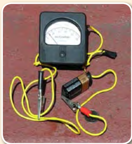
Figure 1b: Homemade water level indicator device consisting of 9V battery, micro-ammeter, two leads (red and black) from the back of the meter, battery connector, four washers, and alligator clips in order to attach one to the casing and other to the bared upper-end of a sounding wire.
