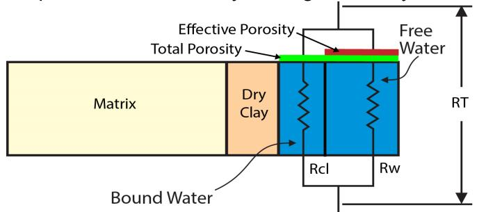
Conductance of electrical current through a wet sand is modeled as a parallel-conductor circuit, one path through the formation water and another through water associated with the clays.
