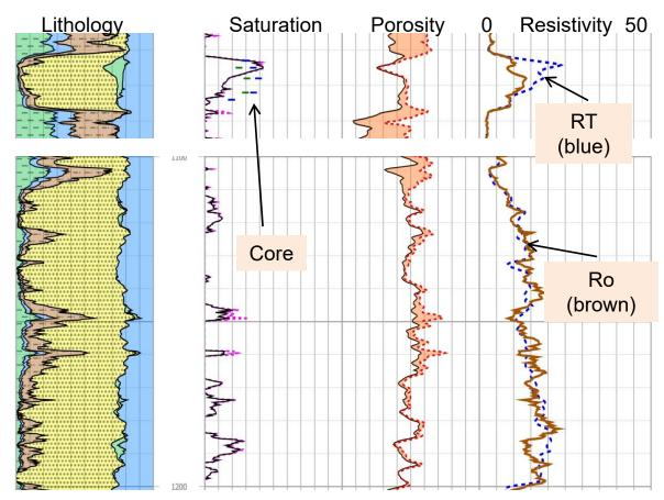
Clay parameters were established in the upper oil-bearing sand by matching the Sw from the full WS model to the core points. These clay parameters were then applied to the suspected wet sand below. It was discovered that the sand actually has some thin intervals of residual oil saturation.
