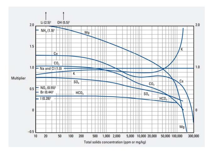
This chart allows the apparent TDS as NaCl to be calculated for a water with significant amounts of other ions present. The Rw of the water can then be determined from the NaCl chart.
