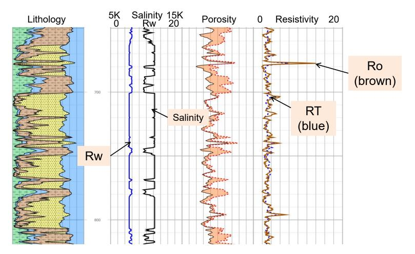
Water from this interval tested at about 10,500 ppm TDS. The Rw values from analysis that provide the best match between Ro and RT correspond to an apparent NaCl salinity of about 11,150 ppm TDS.
