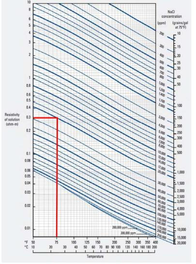
Conversion approximated by  $R_2 = R_1 [(T_1 + 6.77)/(T_2 + 6.77)]^\circ F$  or  $R_2 = R_1 [(T_1 + 21.5)/(T_2 + 21.5)]^\circ C$
