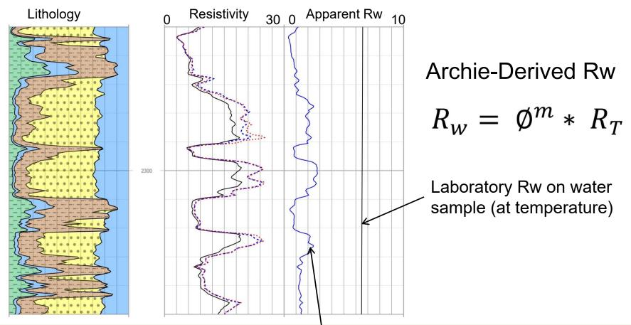
Apparent Rw from a simple Archie analysis (blue curve) is much lower than Rw measured in the laboratory on a sample taken from this zone (black line). Apparent TDS calculated from the Archie-derived curve will be too high.
