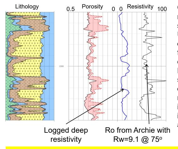
Calculation of Ro is a good model validation step, since Ro should equal RT in wet sands. Using lab Rw value of 9.1 ohm-m @75° (adjusted to formation temperature) with no clay correction, the calculated Ro is about 55-65 ohm-m in sands (black curve). Log derived deep resistivity is much lower, about 25 ohm-m in the sands. This difference indicates that clays are affecting the results.
