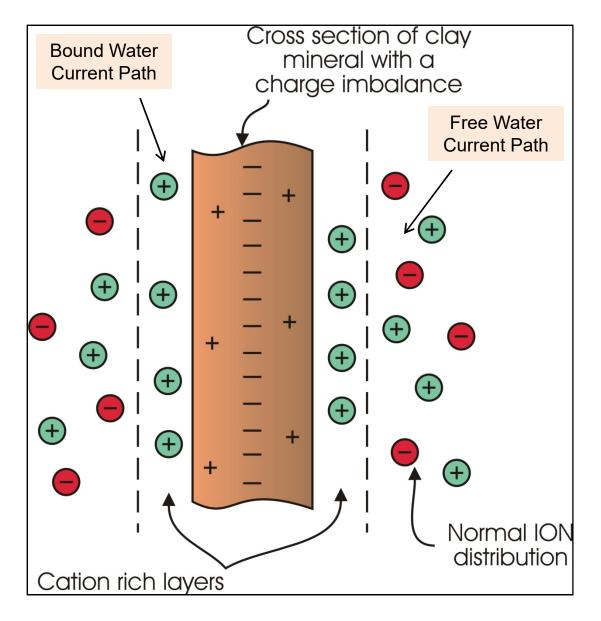
The clay surface has a net negative charge and many charge sites that must be balanced by counterions (cations) that are in equilibrium with the cations and anions in the formation water, lons move between the clay water and the free water. Though a simplification of reality, one can think of two current paths located within the bound water and free water (illustrated left).
