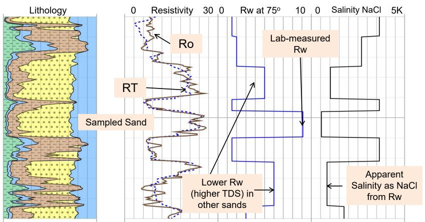
The water resistivity curve (variable by zone) required to calculate the Ro curve from the Waxman-Smits model is shown as the blue curve. Labmeasured Rw of 9.1 ohm-m provides a good answer in the sand at 2296' but lower Rw values (higher salinity) were needed in the other sands. The water sample must have come from the 2296' sand.
