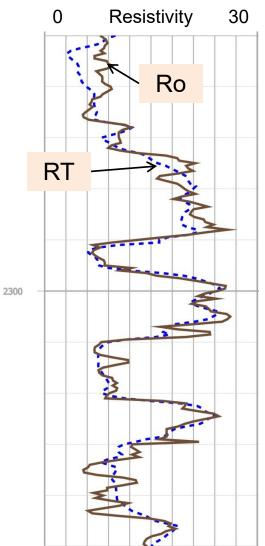
When Ro is calculated using the complete clay correction model, it is possible to achieve a very close fit between the computed Ro and the logged RT.
