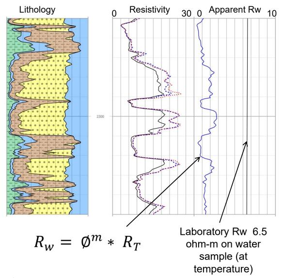
If there were no clay conductivity included in the logged resistivity, the apparent Rw calculated from the simple Archie formula would be all that was needed. But clearly, even though total clay volume is 4%-7% in these sands it contributes significant conductivity, shown by the Rwa values so much lower than the measured Rw. TDS therefore will appear to be too high.
