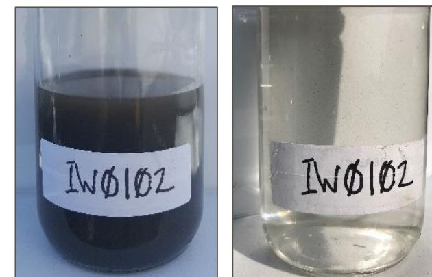
IW0102 water before & after back-flushing
